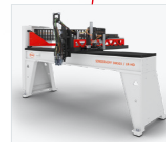
Highly efficient LR-HD 3-axis linear robot for precise guidance of mixing heads for the application of polymer reaction materials. The rack and pinion drive with high stiffness and acceleration enables dynamic application speeds.
