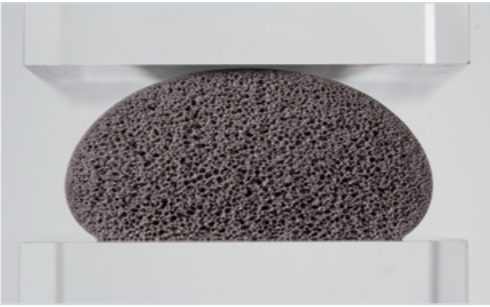
The unpressed polyurethane foam gasket before installation.
